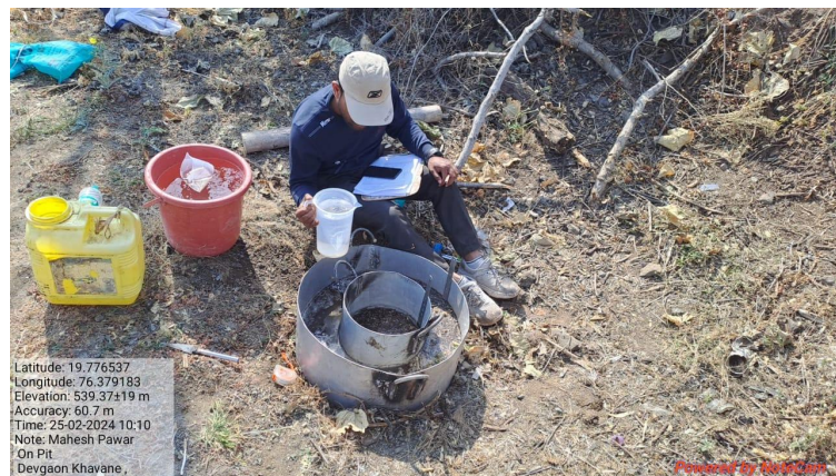
Figure 23a (left): Double-ring infiltrometer experiment on pit where top-of-pit infiltration was the lower than the on-farm infiltration rate (pit #5). Figure 23b (right): Infiltrometer experiment on pit where top-of-pit infiltration was same or higher than the on-farm infiltration rate (pit #8).
