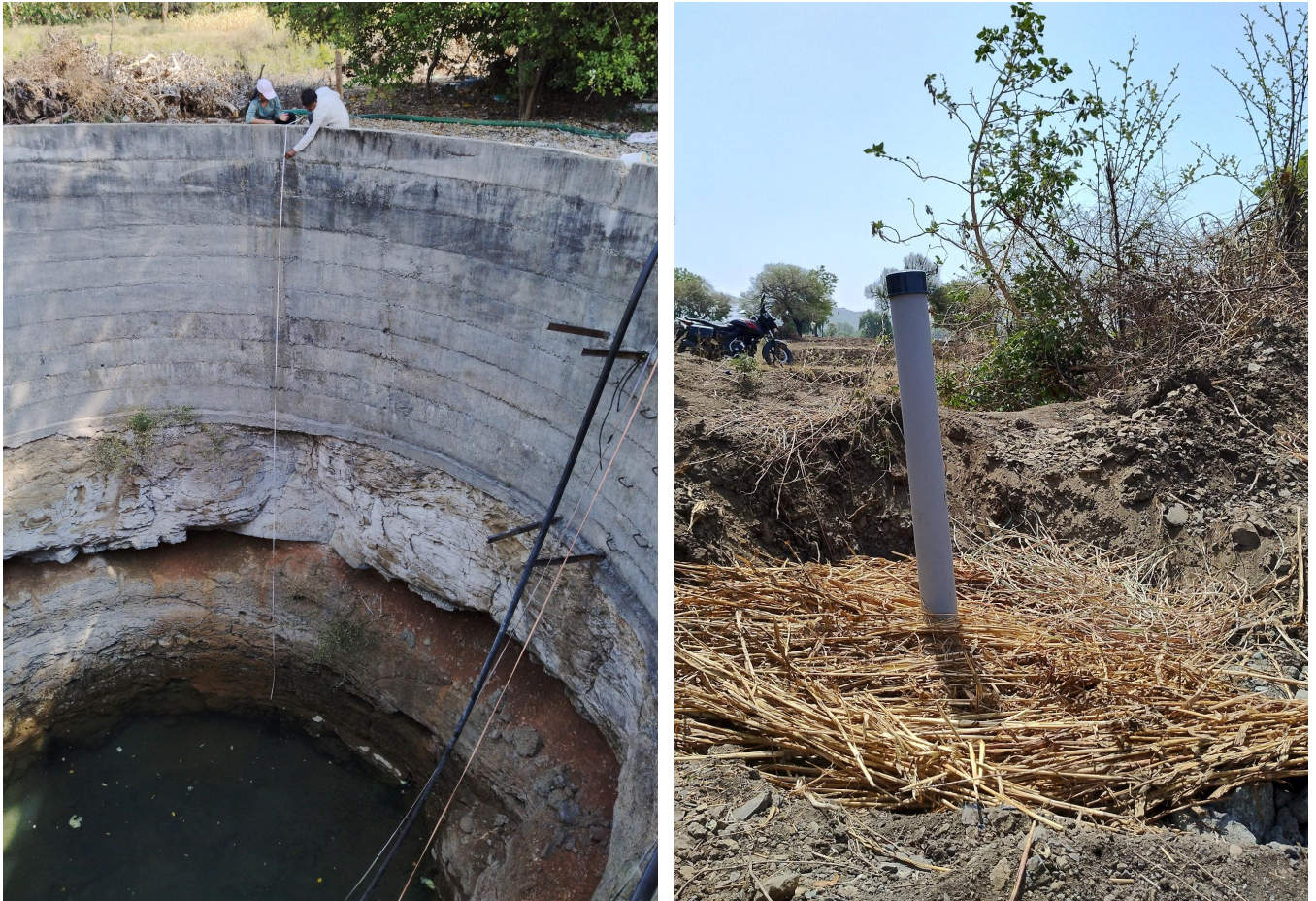
Figure 38a (left): Field researchers taking pre-monsoon static water-level measurements in a well located in a paired watershed. Figure 38b (right): Perforated PVC pipe installed in the modified pit design implemented in a farm for measurements with a pressure transducer for further tests.
