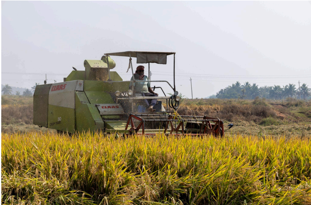
Figure 5: Paddy harvest in BR Gunda village, Raichur district. A combine harvester takes only an hour to harvest an acre of paddy. Photo by Nabina Chakraborty
