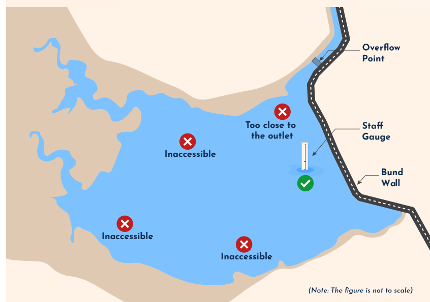
Figure 1: The staff gauge should be placed in an appropriate location in the water body.
