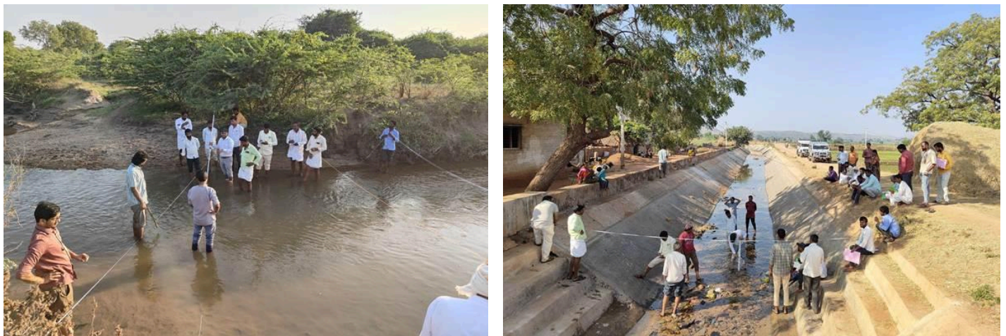
Figure 8: Stream cross-section and depth measurement (left); Canal cross-section and depth measurement (right)
