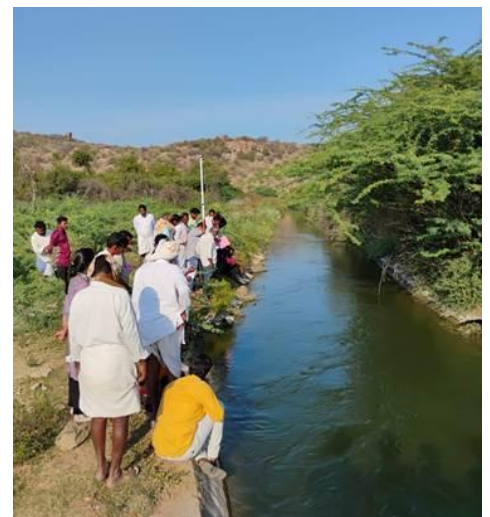
Figure 9 (right): Measuring water velocity using the leaf-and-stopwatch method
