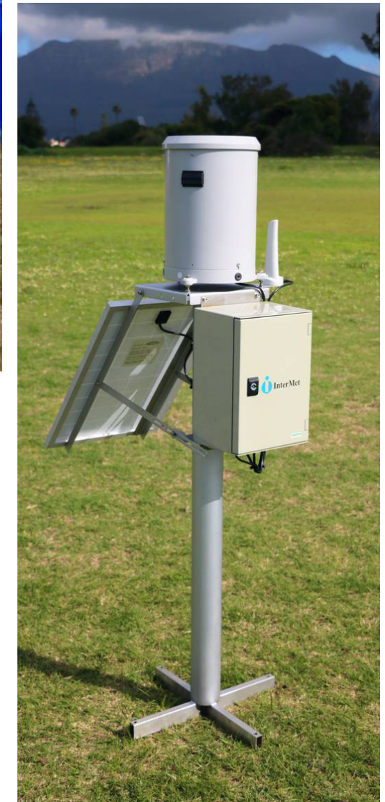
1.29. Automatic rain gauge
